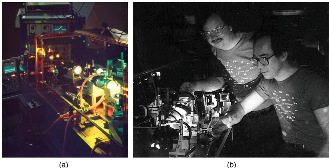
▲ **Fig. 3.** The first femtosecond laser, a Rhodamine 6G dye laser passively mode-locked by a DODCI saturable absorber dye. (a) Instruments record the pulse train and a sub-picosecond-resolution pump-probe trace of a molecular response. (b) Chuck Shank and Erich Ippen with their laser.
