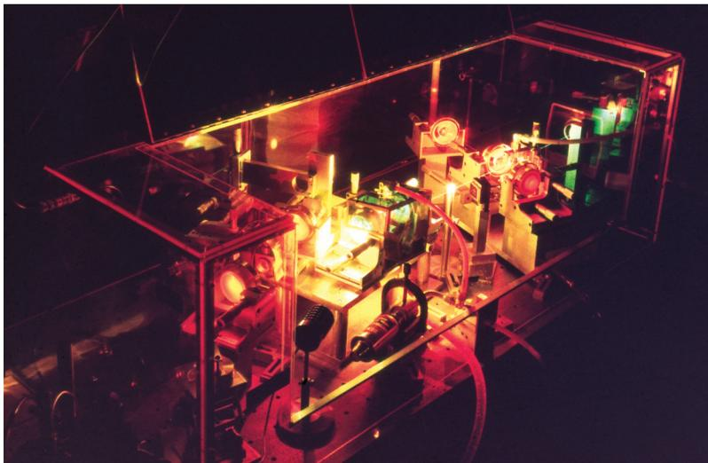
◀ **Fig. 4.** High power, 3-stage, femtosecond dye laser amplifier pumped by frequency-doubled Nd:YAG laser at 10 Hz.
