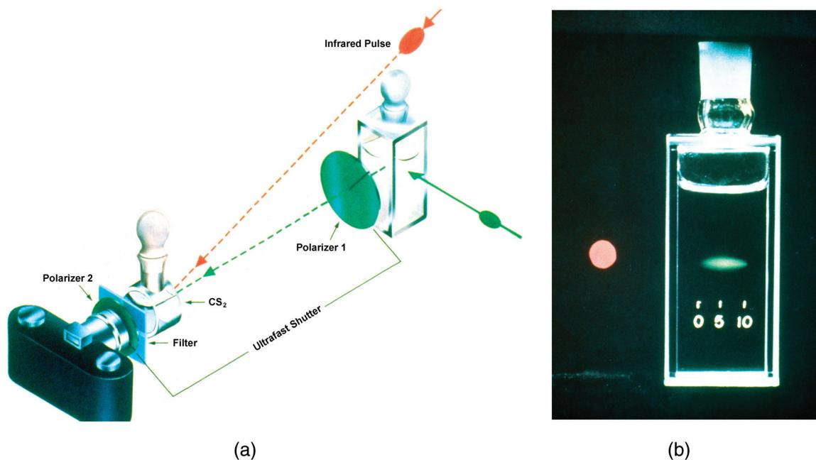
▲ **Fig. 1.** Light in flight. An optical Kerr effect shutter, operated by a picosecond infrared pulse, is used to capture the image of a picosecond pulse passing through a lightly scattering liquid. (a) experimental arrangement (b) the photo. Reprinted with permission from M. A. Duguay and J. W. Hansen, *Appl. Phys. Lett.* **15**, 192–194 ©1969, AIP Publishing LLC.
